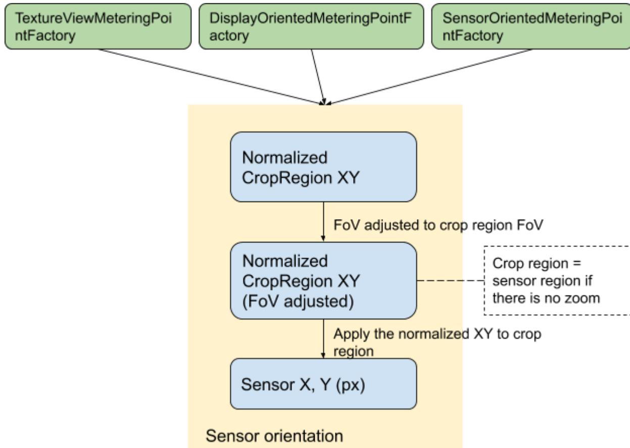
The Above diagram illustrates the main flow of the coordinates translation. The 3 MeteringPointFactory we introduced in previous section will all convert to the **normalized XY in crop region** and then follow the same procedure to be translated to the final sensor coordinates. Let's explain some steps below:
