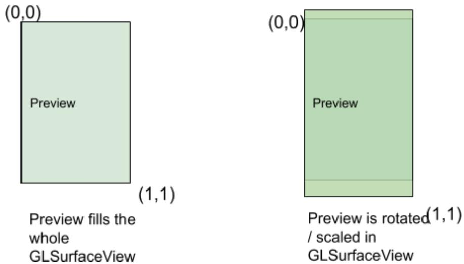
CameraX translates the normalized view points to the normalized crop region XY by using the display orientation , the sensor orientation and front camera mirroring. The reason CameraX uses display orientation instead of the rotation degree returned in Preview#OnPreviewOutputUpdateListener is because the View XY has the same orientation as the display orientation.
